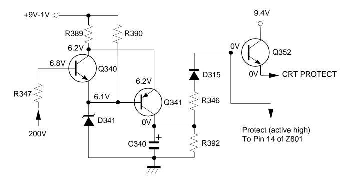
Figure 17-14 200V Under Voltage Protect Circuit (Located on Convergence Out/Power2 Board)
