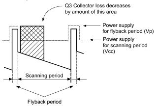
Fig. 11-7 Output stage power supply voltage
