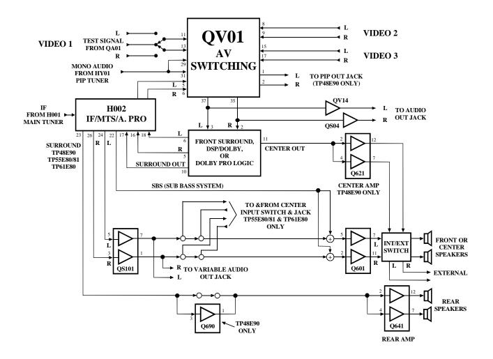
Figure 1-8 Audio Signal Flow Block Diagram
