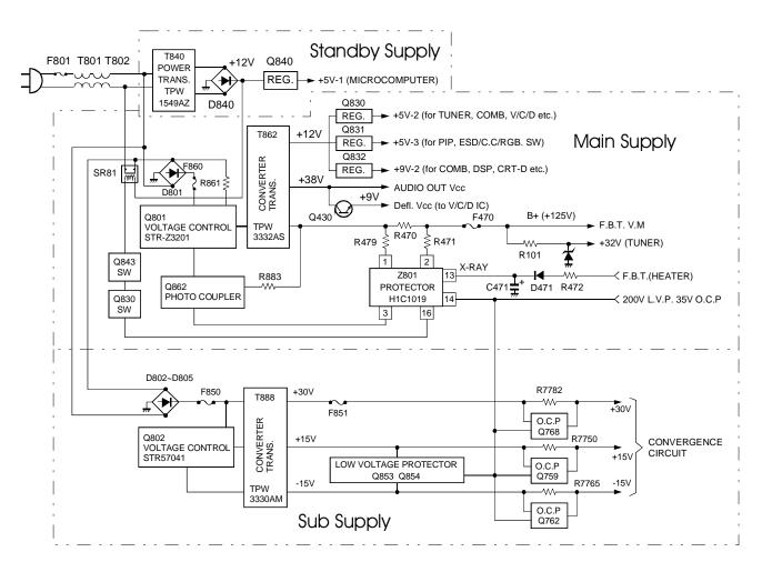
Figure 17-1 Power Supply Block Diagram
