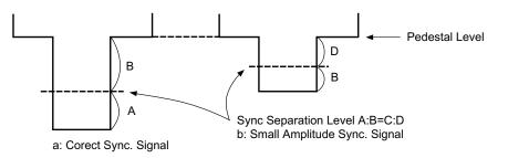
Fig. 10-2 Synchronous separation by auto slider system
