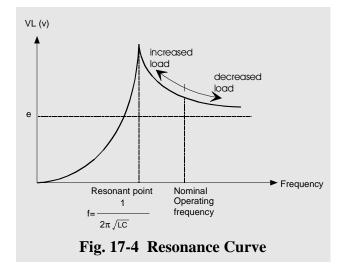
increases. Conversely, when the load decreases, the frequency increases and the current decreases. Table 17-1 shows the voltages developed on T862 secondaries.
