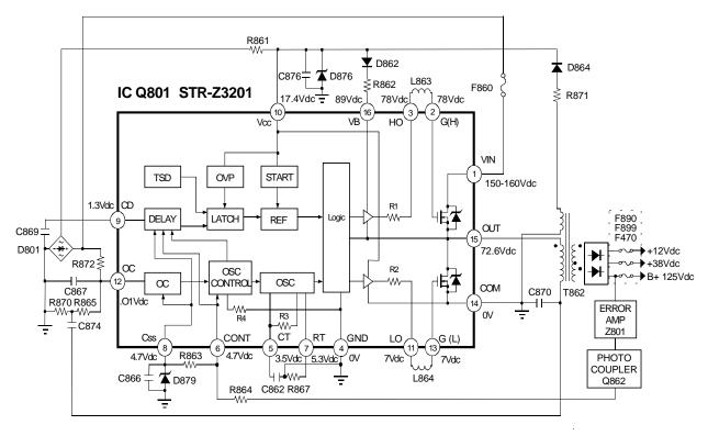
Figure 17-3 Current Resonant Supply (Main)
