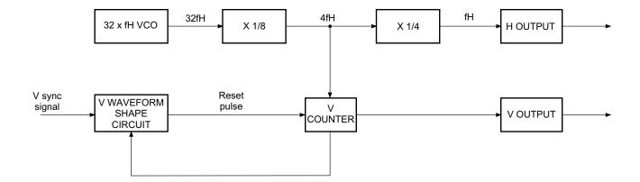
Fig. 10-6 Block diagram of H, V count down circuits
