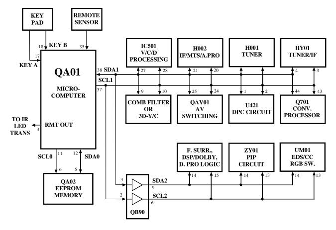
Figure 1-11 I<sup>2</sup>C Communication Block Diagram
