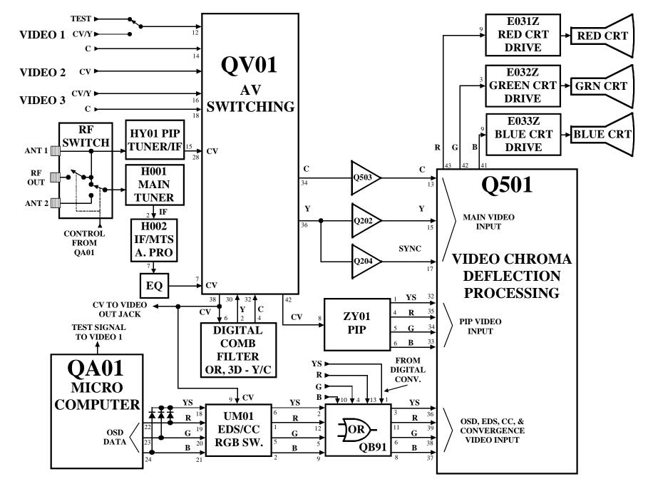
Figure 1-7 Video Signal Flow Block Diagram
