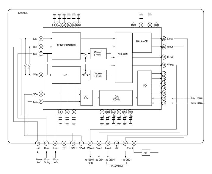
Fig. 2-3 A.PRO block diagram
