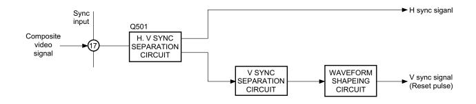
Fig. 10-1 Sync separation circuit block diagram
