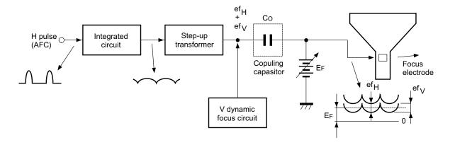
Fig. 18-1 Block diagram of H dynamic focus circuit
