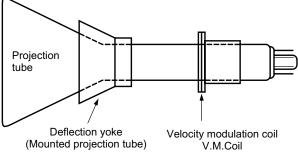
Fig. 16-14 Mounting position of deflection yoke and V.M coil
