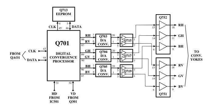
Figure 1-13 Convergence Block Diagram
