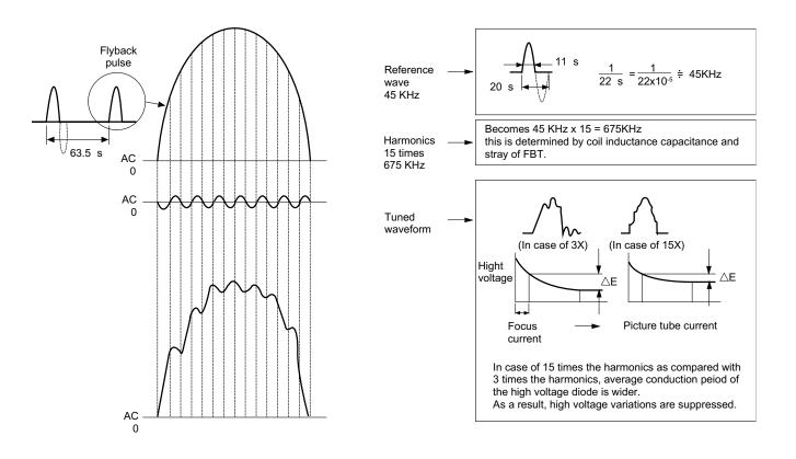
Fig. 12-21 Tuned waveforms
