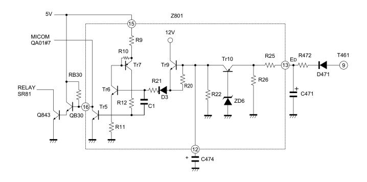
Fig. 12-26 X-RAY protection circuit
