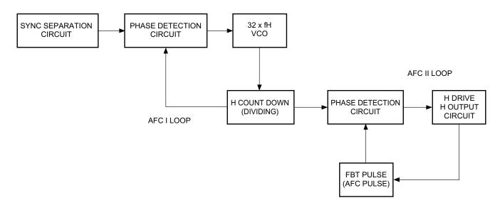
Fig. 10-3 H AFC circuit block diagram
