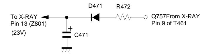
Figure 17-15 X-Ray Protect Circuit (Located on Deflection/Power Board)
