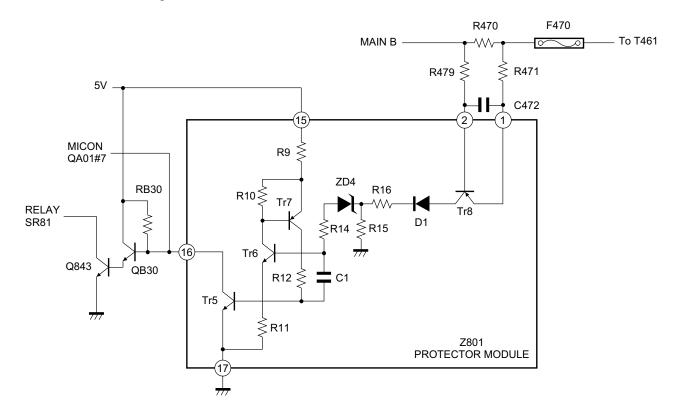
Fig. 12-27 Over current protection circuit
