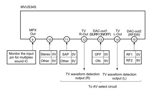
Fig. 2-2 Block diagram of MVUS34S
