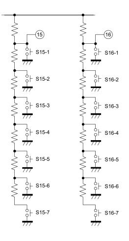
Local key detection in the N5SS chassis is carried out by using an analog voltage divider-like method which detects a voltage appearing at the local key input terminals (pins 17, 18) of the microcomputer whenever a key is depressed. Using this method, a maximum of 14 keys can be interpreted.
