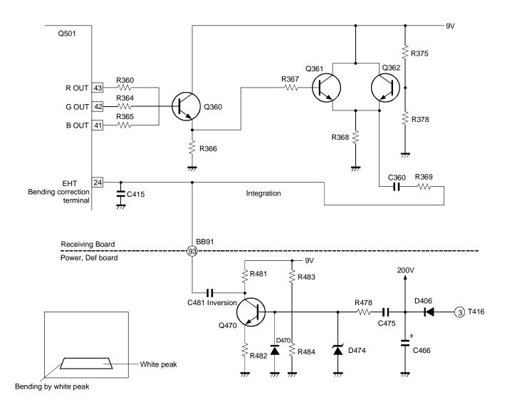
Fig. 12-13 White peak bending correction circuit
