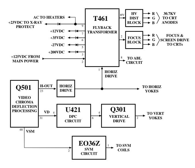
Figure 1-10 Horizontal and Vertical Deflection Block Diagram
