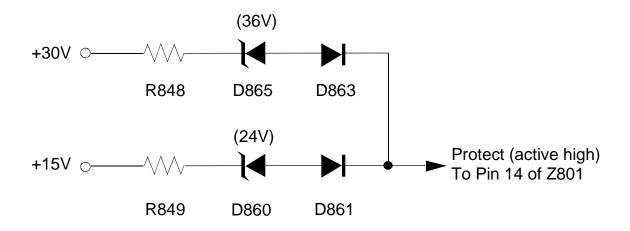
Figure 17-12 +30V/+15V Over Voltage Protect Circuit (Located on Convergence Out/Power2 Board)
