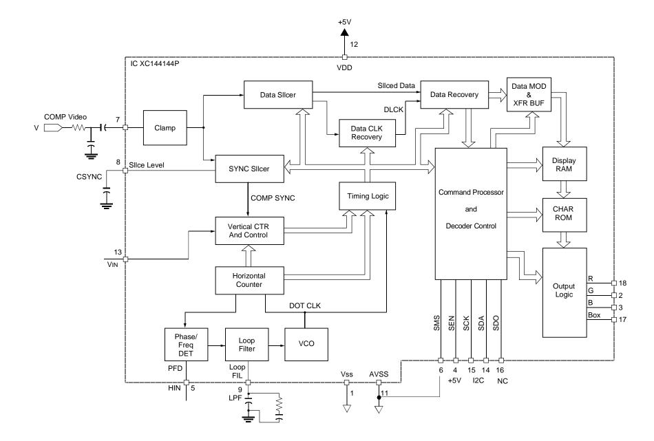
Fig. 14-5 XC144144P QM01 block diagram
