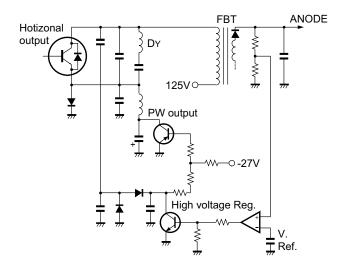
Fig. 12-22 Basic circuit for high voltage regulator emplyed in the unit
