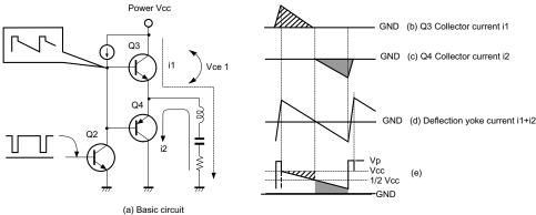
Fig. 11-6 Output stage operation waveform
