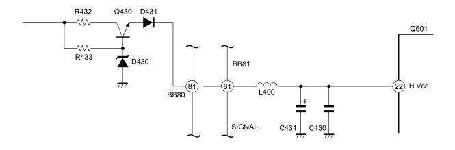
Fig. 12-1 H drive circuit block diagram
