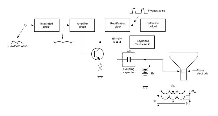
Fig. 18-3 Block diagram of V dyanamic focus circuit
