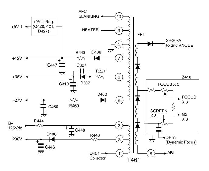
**Figure 17-6 Scan Derived Sources**
