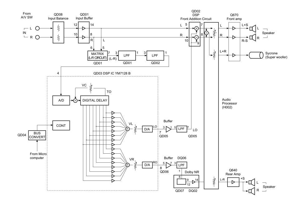
Fig. 5-3 Block diagram of DSP circuit
