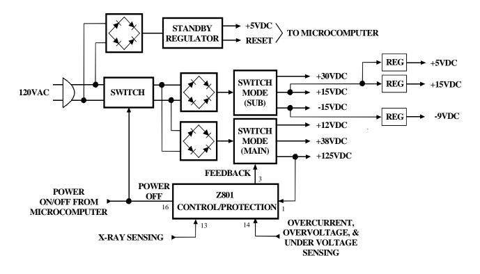
Figure 1-9 Power Supply/Protection Block Diagram
