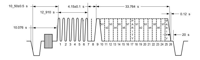
Fig. 14-1 Line 21 waveform
