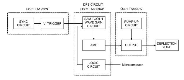
Fig. 11-1 Block diagram of V deflection circuit
